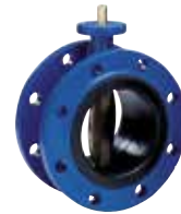
Series 75/20 Centric butterfly valve with fixed liner Double flanged short Ductile iron DN 50-2000 With any type of actuation
