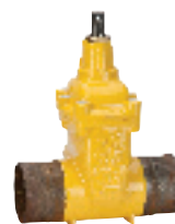
Series 46/64 Gate valve with short spigot ends DN 50-300 PN 16 GS-C 25 N With external epoxy coating
