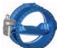
Series 756/102 Butterfly valve Double eccentric Double flanged Stainless steel seat ISO-input gearbox DN 200-2800 PN 10/16 Ductile iron
