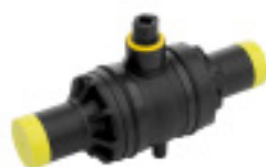
Series 85/50 Ball valve with spigot ends DN 16 / Ø 20 mm - DN 150 / Ø 180 mm PN 10 PE 100
