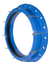
Series 260 Fabricated coupling for AC, steel, cast iron and ductile iron pipes Steel DN 350-2000 PN 10/16/25
