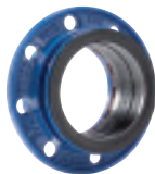
Series 05 Combi-flange for D.I. pipes Non-tensile DN 50-600 Tensile DN 50-300 PN 10/16 Ductile iron
