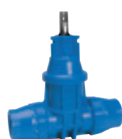
Series 16/50 Service connection valve with tensile socket ends for PE pipes DN 25-50 PN 16 POM (Polyoxymethylene)
