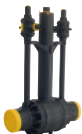
Series 85/50 Ball valve with spigot ends, stem extension and 2 purge points DN 50 / Ø 63 mm - DN 150 / Ø 180 mm PN 10 PE 100
