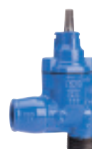
Series 11/30 Service connection angle valve with external thread on inlet and tensile socket end for PE pipes on outlet DN 25-50 PN 16 Ductile iron
