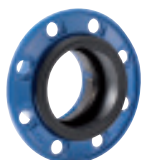
Series 05 Combi-flange for PE and PVC pipes Non-tensile (PVC) DN 50-600 Tensile DN 50-300 PN 10/16 Ductile iron
