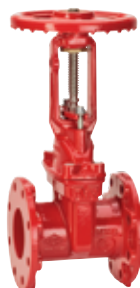
Series 145/46 Flanged gate valve with rising stem dedicated to UL and FM requirements 250 PSI DN 65-200 Ductile iron UL/ULC listed, FM approved
