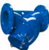
Series 910 Y-strainer DN 50-300 PN 10/16 Ductile iron Stainless steel screen
