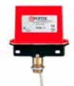
Series 96/00 Supervisory switch for monitoring the position of post indicator valves and series 145 OS&Y valves UL listed FM approved
