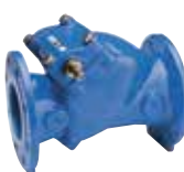
Series 41/60 Swing check valve Resilient seated Free shaft DN 50-300 PN 10 or 16 Ductile iron
