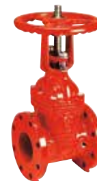
Series 145/46 Flanged gate valve with rising stem dedicated to UL and FM requirements 250 PSI DN 65-200 Ductile iron UL/ULC listed, FM approved
