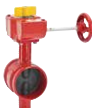
Series 815 Centric butterfly valve Rubber vulcanized disc Grooved ends to AWWA C606 DN 65-200 300 PSI Ductile iron UL/ULC listed, FM approved
