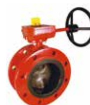
Series 75/41 Butterfly valve Centric with fixed liner Double flanged short DN 50-300 PN 10 or 16 Ductile iron FM approved
