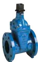
Series 45/59 NRS Flanged gate valve with wrench nut to AWWA C509 DN 50 and DN 250-400 DN 50 and DN 250-300: 250 PSI DN 350-400: 200 PSI Ductile iron UL/ULC listed, FM approved
