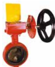
Series 75/10 Butterfly valve Centric with fixed liner Wafer DN 50-300 PN 10 or 16 Ductile iron FM approved
