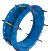
Series 265/30 Fabricated dismantling joint for all pipe materials Steel DN 300-1200 PN 10/16/25
