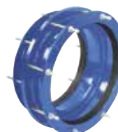
Series 259 Fabricated step coupling for AC, steel, cast iron or ductile iron pipes Steel DN 350-2000 PN 8 to 25
