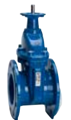
Series 15/42 Flanged gate valve with ISO top flange for actuator Face-to-face DIN F4 DN 40-400 PN 10/16 Ductile iron
