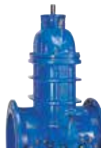
Series 55/30 Flanged gate valve DN 450-500-600-800 Face-to-face DIN F5 PN 10/16 Ductile iron Resilient seated Replaceable stem sealing
