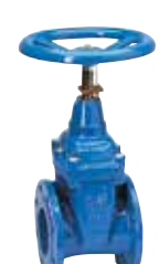
Series 06/35 Flanged gate valve with pin indicator Face-to-face DIN F4 DN 50-400 PN 10/16 Ductile iron
